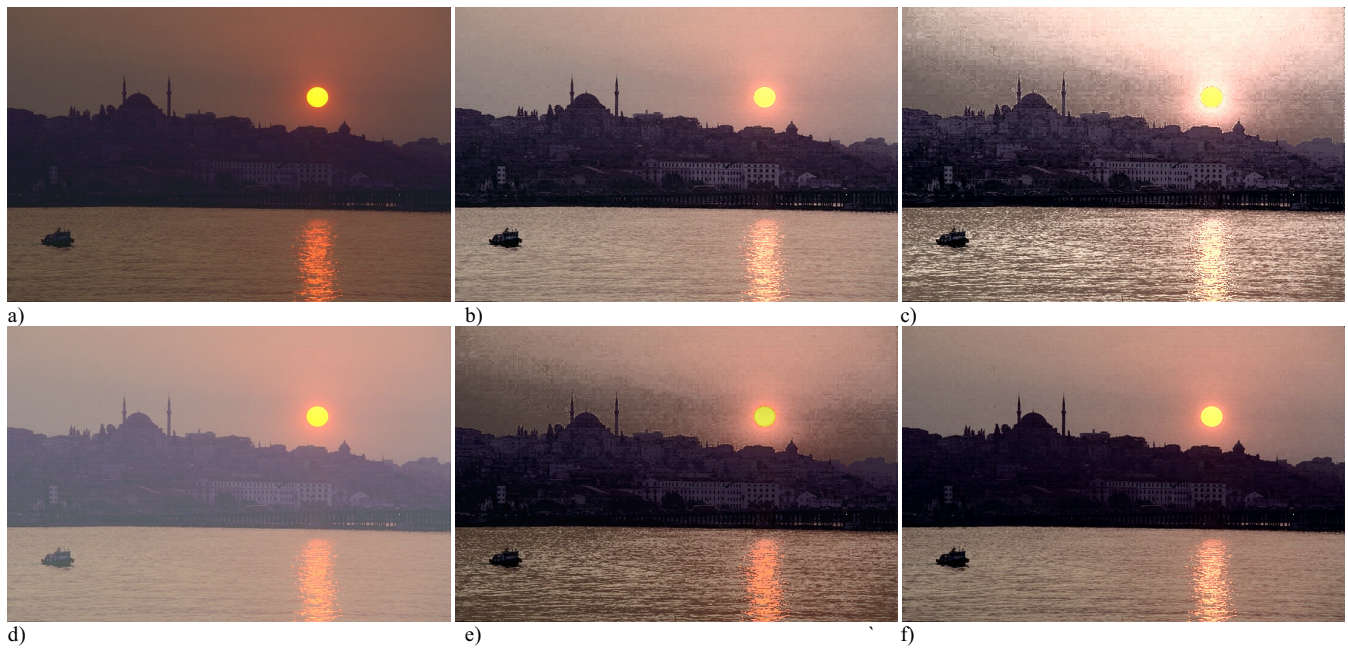
Fig. 4. The enhancement results for test image Scene , a) original image, b) output of the proposed approach, c) output of histogram equalisation, d) output of gamma correction, e) output of PBDHE, f) output of DRSHE.
